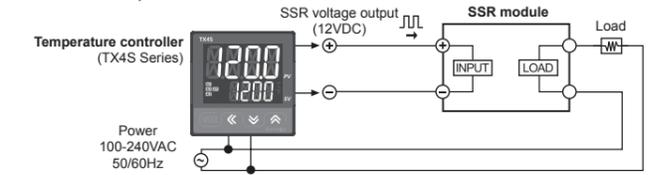
※When selecting cycle or phase control mode, the power supply for a load and a temperature controller must be the same.
