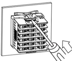
Mount the unit on the panel. Push the bracket with tools to fix the unit as the figure.
